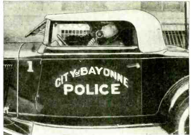
The photo above shows 8.6 meter combination "transmitter-receiver" installed in police car.
