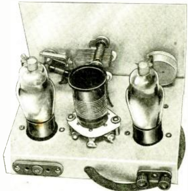
Rear view of the 2-tube "Pentaflex" receiver, designed by Mr. Worcester of "Oscillodyne" fame.
